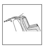
If the position you are using does not have a head restraint and you are using a dual tether, route the tether over the seatback.
